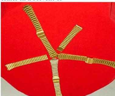
Figure 13. TiN /Au coated watch straps
